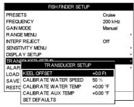
Figure 17.12 - Transducer Setup menu
